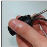
(1) Verify the position of 'TOP' which should be upper side and fix it to the lens bracket with screws.
