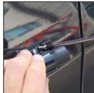
(4) Fix the pre-installed camera using the rubber packing and screws.
